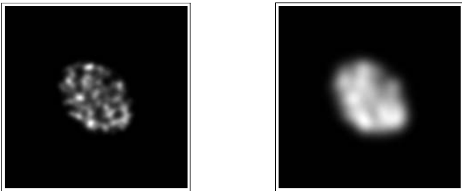
Fig. 10. At left the product of the blurred point sets (the “correlation blur”), at right the “blurred correlation blur”. The blurred correlation blur is a good estimate of the “overlap” defined by the “overall shapes” of the point clouds.
